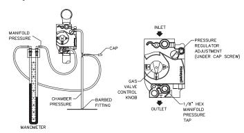
FIG. 31 Measuring Manifold Gas Pressure
